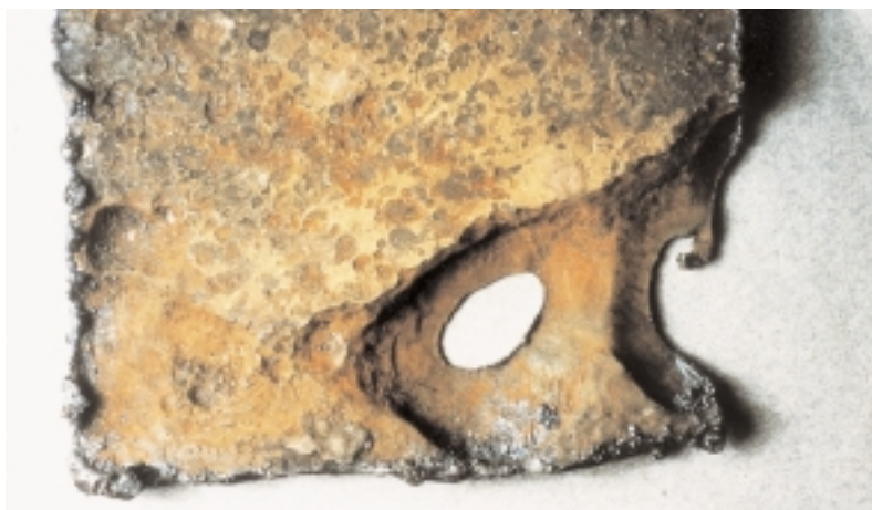
The above is typical sulphate reducing bacteria (SRB) corrosion pitting of a diesel oil storage tank 10 mm bottom plate which occurred within nine months.
